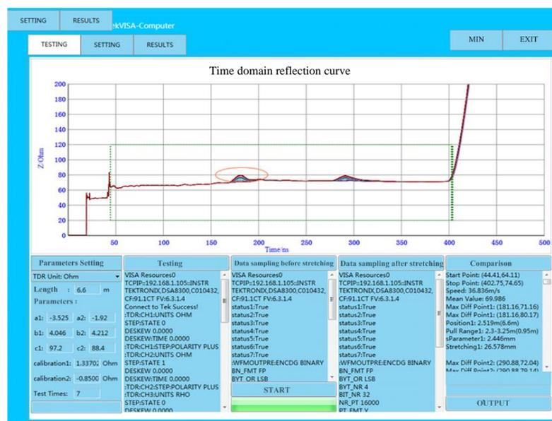
**Figure 8.** Software interface for the distributed measurement of deformation based on the TDR technique.
